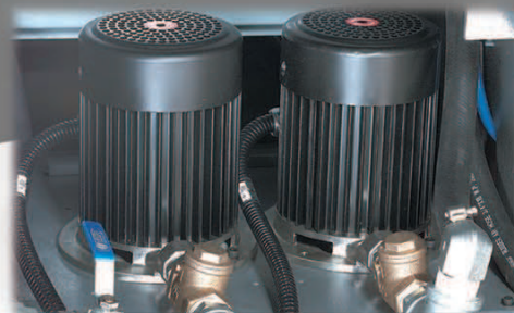
Dual vertical coolant pumps 直立式泵浦
