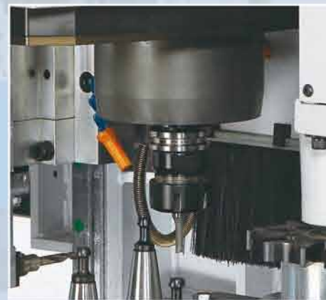
C-AXIS ROTATION MECHANISM C 軸旋轉機械結構
