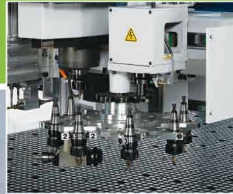
DRUM TYPE AUTO. TOOL CHANGE SYSTEM 圓盤式換刀系統
